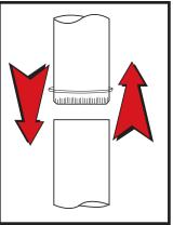
• Secure each joint between sections of chimney connector, including telscoping joints, with at least three sheet metal screws. The pre-drilled holes in the top of each section of
